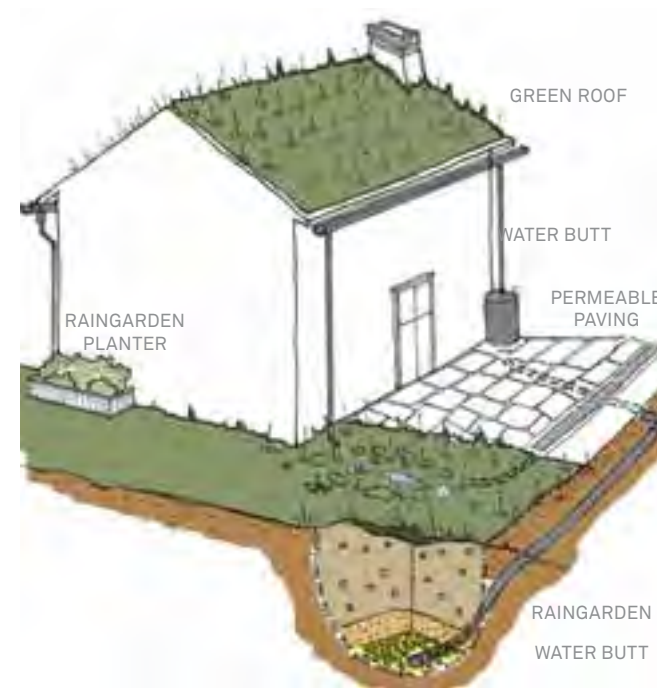
Figure 3.127 Diagram showing various source control measures at property level and connections to wider system
