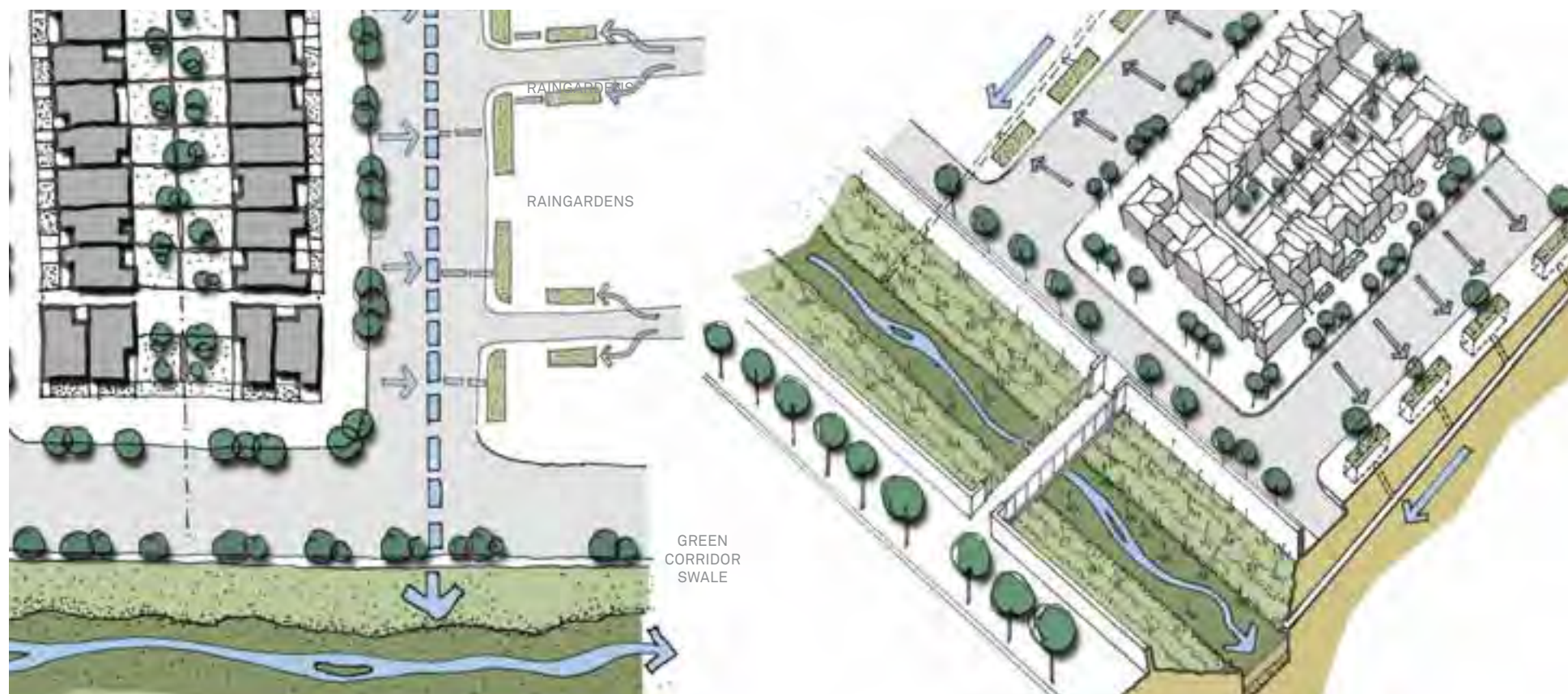
Figure 3.128 Hierarchy of streets, swales and Green Corridors, aiming to use overland flow where possible to avoid deep pipes and deep receiving swales
