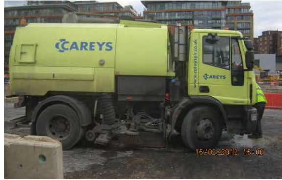
Figure 5 Example of watering haul road to suppress dust and road sweeper
