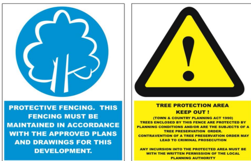
Plate 10: Example of Tree Protective Fencing sign
