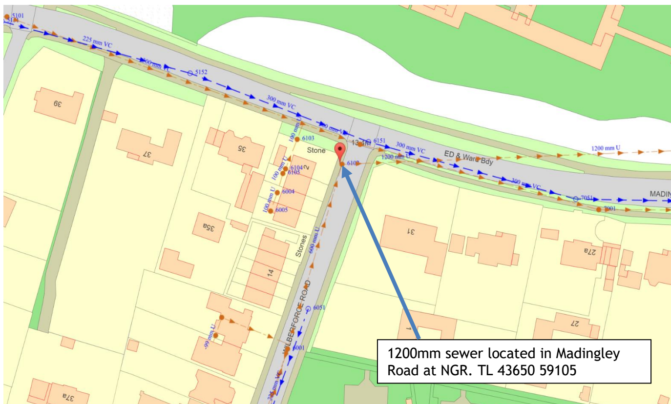
Figure 1: Showing your connection point for foul water
